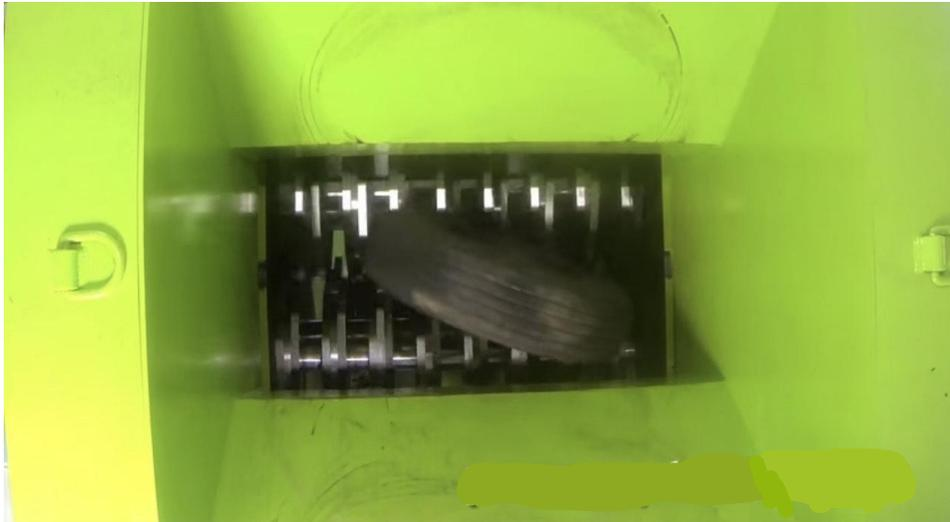
Figure 3. A double shaft tire shredder. Source: (Eco Green).
