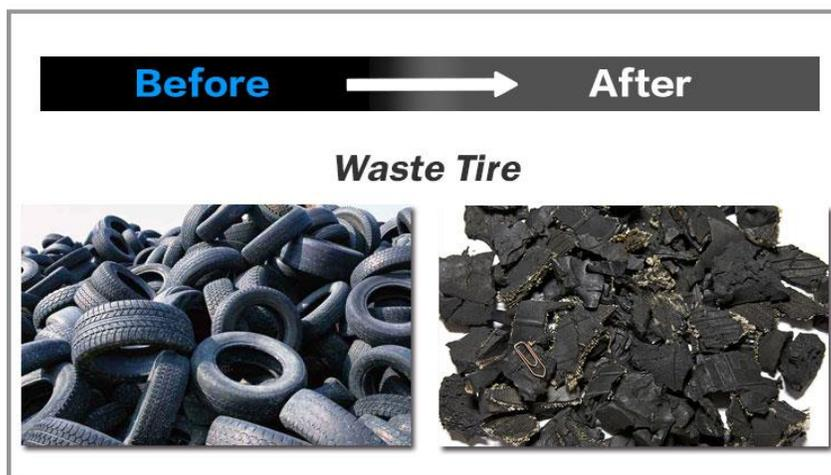
Figure 1. Whole tires before and after they are shredded into TDA (Wanrooe, 2019).
