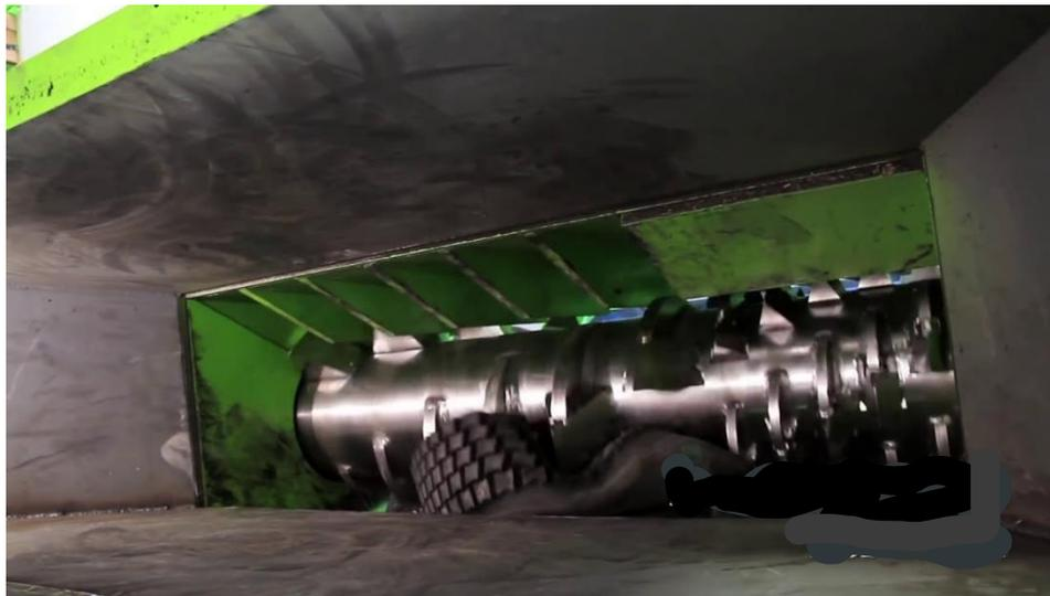
Figure 2. A single shaft tire shredder. Source: (Eco Green).
