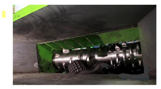
Figure 2. A single shaft tire shredder. Source: (Eco Green).
